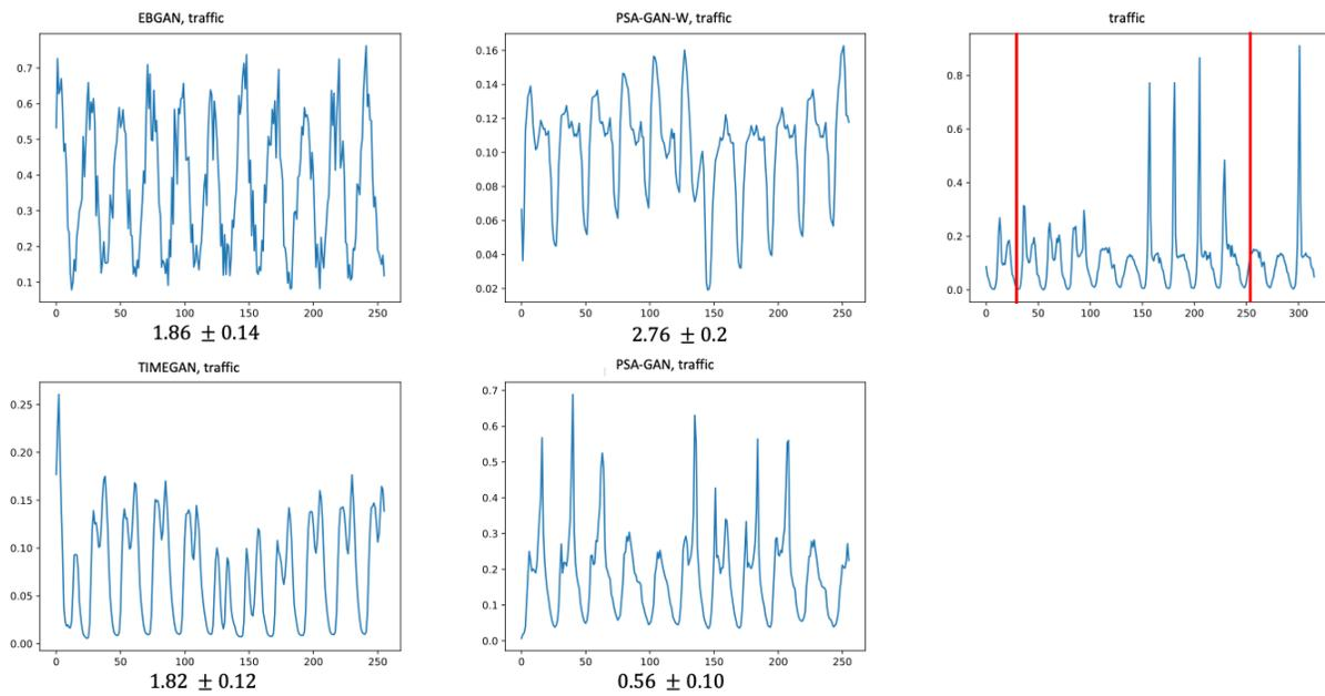
Figure 3. Time Series - Traffic: On the left we plot four synthetic time series at the same time range. On the right we plot between two vertical red line a real time series at the same time range. On the left and right of the red lines is the context of the real time series, 30 time points before and after. We also show the FID score for each model.
