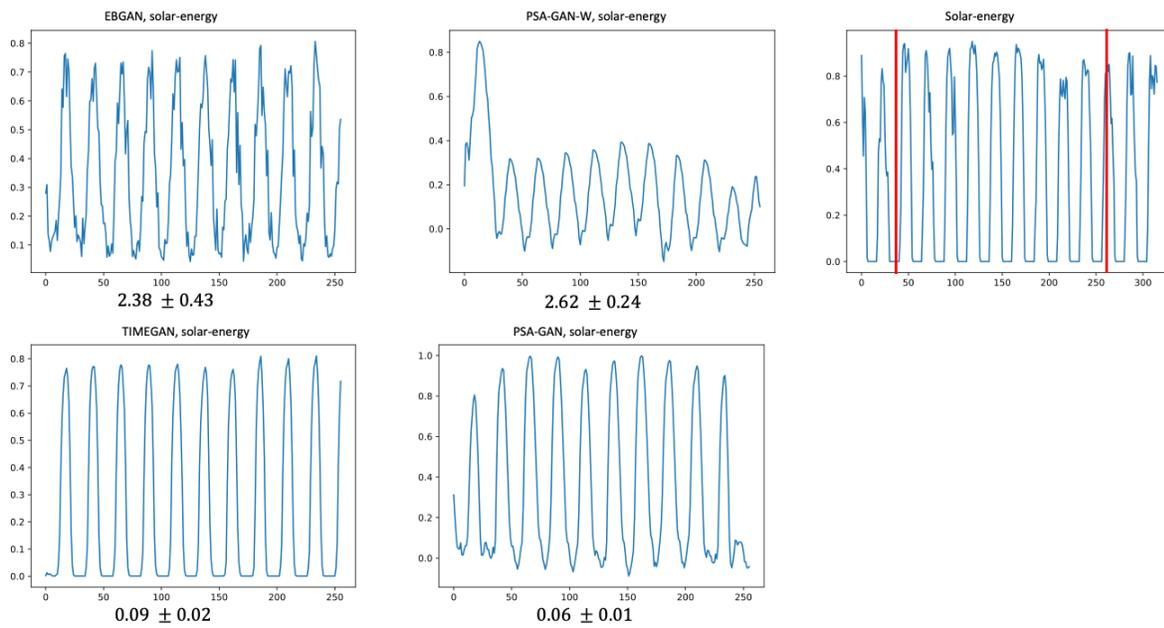
Figure 1. Time Series - Solar-Energy: On the left we plot four synthetic time series at the same time range. On the right we plot between two vertical red line a real time series at the same time range. On the left and right of the red lines is the context of the real time series, 30 time points before and after. We also show the FID score for each model.
