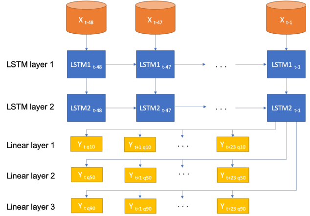
Figure 2. The architecture of our LSTM model. We use multi-step LSTM to forecast multiple horizons. The input is two-day data of size 48 \times 44 and the output is the prediction of three quantiles of next one-day electrical load values.
